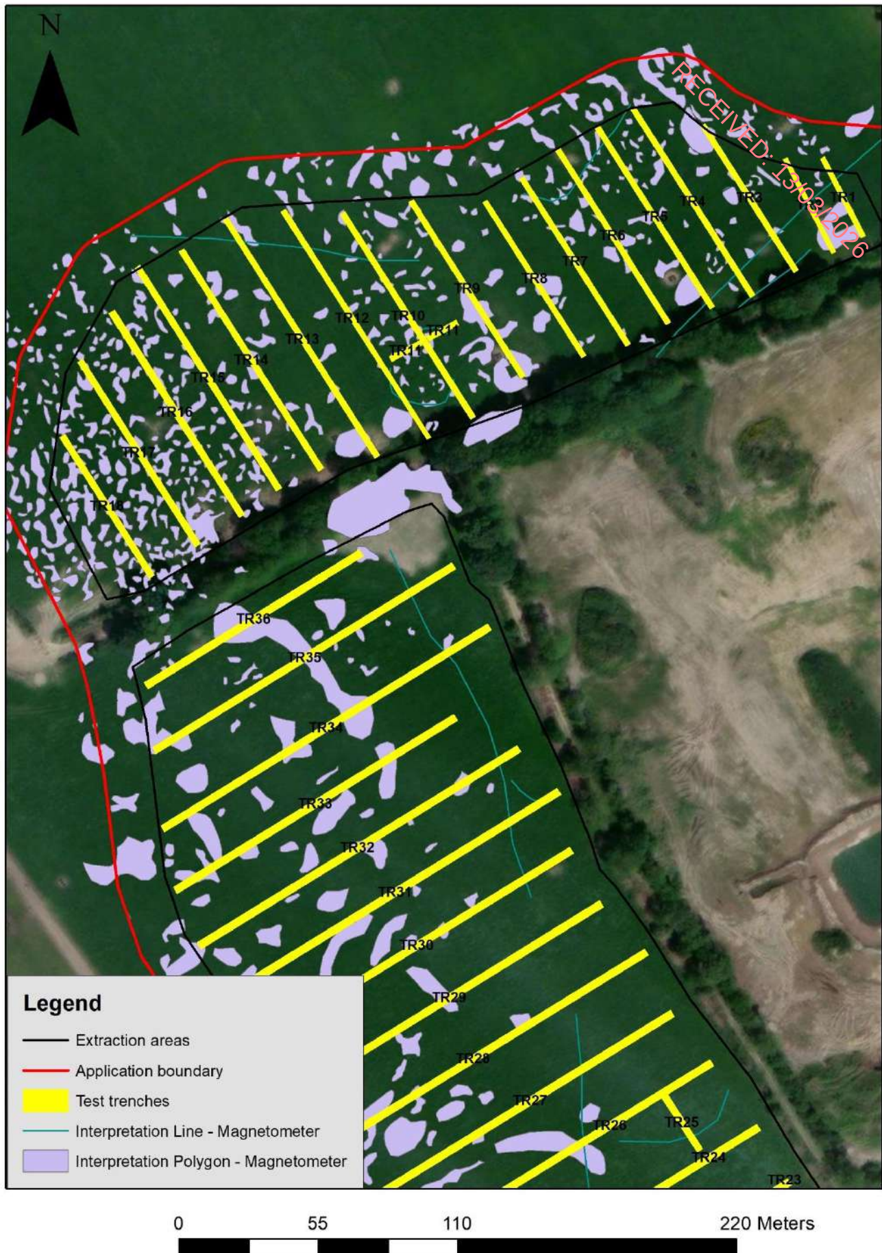
Figure 8: Trench layout in relation to geophysical anomalies (please see geophysical survey report for detail of anomalies).
